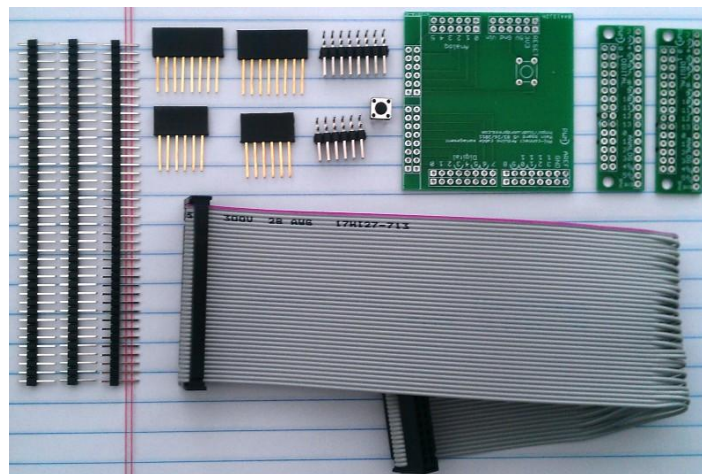
Fig. 2 Phi-connect kit parts. Picture has connector boards V1.8 (top right).
