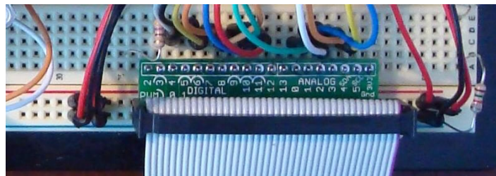
Fig. 5-2 Insert breakout board on a breadboard per picture. Make sure that you have inserted the downward 2-pin firmly into the busses on the side of your board. This powers these busses and stabilizes the breakout board.
