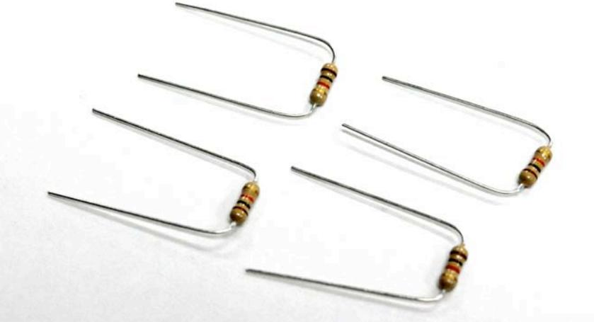
Figure 2: After bending the resistor leads
